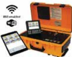
The Model 6600-NG Automated Tester is designed to test aircraft equipped with SmartProbes™. The tester has one Static output (Ps1), one Pitot output (Pt) and a third output (Ps2) which can be used to simulate either AOA (angle of attack) or AOS (angle of sideslip). Using the small and light-weight Remote, an operator can test the entire pitot and static system from the cockpit. The Model 6600-NG comes with a removable 8-hour battery (optional),
