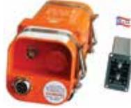
GPS capable ELT accepts Garmin aviation, Bendix/King aviation, NMEA 0183 and Arinc 429 data. Retains GPS coordinates after power is removed. Remote fits Artex and Kannad panel cut-outs. ELT certified to the new TSO-C126B standard battery certified to TSO-C142A lithium batteries UN/DOT 8.3 lithium batteries.
