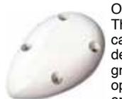
Operates with all new WSI InFlight® capable receivers. The antenna receives Sirius Satellite Radio broadcasts to enable the WSI weather service. It was designed specifically to suppress interference from ground based signals. Its proprietary design allows for optimum performance while the aircraft is turning. The antenna has been thoroughly tested and meets all of the RTCA DO-160E requirements.
