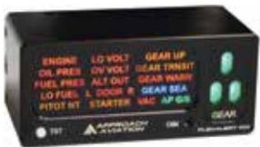
The FlexAlert Multifunction Annunciator is an all-in-one multifunction display that places critical warning and condition annunciations directly in front of the pilot to increase safety and simplify panel layouts. The sunlight-readable & dimmable LED display includes Landing Gear Status for both
