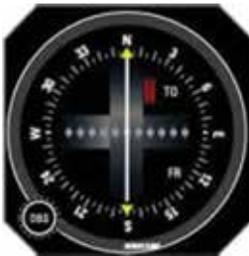
The KI203, KI208, KI204, & KI209 indicators feature an internal VOR/ LOC converter and are compatible with the KX155 transceiver. The KI203 & KI204 have rectilinear meter movement, while the KI208 & KI209 feature pivot needle action. The KI206 has rectilinear meter movement and works with the KX165 & KNS80. The KI209 includes GPS interface capability. Size: 3.125" x 8"D; Weight: 1.5lbs.
