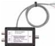
**RAMI ANTENNA DIPLEXER SWITCH / 50 OHMS - AV-590** - The AV-590 diplexer allows two communications radios to share one antenna. In normal, non-switched mode the AV-590 evenly splits the signal between two radio receivers. When the control voltage is activated by a microphone's PTT, the AV-590 switches the antenna to the corresponding radio transmitter and isolates the other receiver. P/N 11-14047 ..... **\$322.00**
