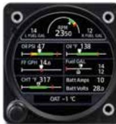
The GI 275 EIS variant can serve as a primary EIS display for piston engine, fuel, electrical and other data. Use dual GI 275 displays to monitor twin-engine aircraft. Graphical display of cylinder head and exhaust gas temperatures allows you to pinpoint the optimal fuel/air mixture for efficient power management.
