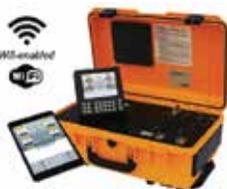
The Model 6300 is a versatile 2-channel RVSM Pitot Static Tester targeted for General Aviation; all Business Jets and Commercial Aircraft. It is used to perform leak-checks and accuracy checks on the Pitot Static systems of RVSM aircraft up to 690 knots & 60,000 ft. Accuracy checks are typically performed on altimeters, airspeed indicators and VSI's. The Model 6300 is equipped with a Remote unit with
