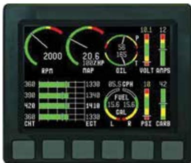
The EMS-D10 is a ergonomically engineered engine monitor that blends traditional analog gauges with newer digital technologies to provide a user-friendly instrument that enhances safety and peace of mind. With up to 27 separate inputs available, the pilot's workload is significantly reduced as the EMS-D10 continuously monitors all sensor inputs for the powerplant, fuel and other miscellaneous systems and immediately annunciates any abnormality requiring attention.
