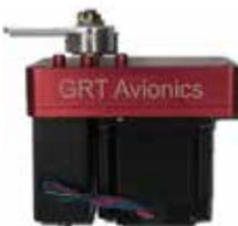
Digital CNC machined servos add autopilot functionality to any GRT Avionics EFIS System. Heading select, VOR/GPS tracking, ILS and GPS precision approach coupling\*, climb/descent to selected altitude using preset IAS or VS\*, automatic approach capture. Pitch servo torque sensing provides Trim Up/Trim Down indication. Clutchless design with shearble output arm provides fail-safe mechanical method of freeing flight controls in the unlikely
