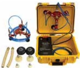
Laversab Universal Adapter for Pitot Static Testers. For most aircraft and helicopters. Customized adapters. Full adapter-kits for specific aircraft. P/N 12-04751
