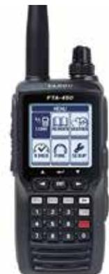
5W TX output. Large 1.7" x 1.7" Dot matrix Display. Back-lit Keypad and Display. 800 mW Audio Output. 200 Memory Channels. 8.33kHz Narrow Band compatible. IPX5 Waterproof rating. Includes High-Capacity 1800mAh Li-ion battery. Includes Alkaline battery tray (6 x AA). NOAA Weather Channels with WX alert. PC programmable.
