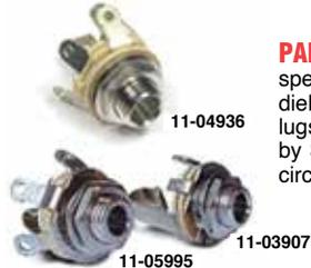
**PANEL JACKS** - Contact springs are of special alloys for long life. Insulation is high dielectric strength phenolic. Tinned terminal lugs for easy soldering. Short frame. Mounts by 3/8-32 threaded bushing and nut. Open circuit until plug inserted.
