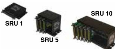
The **SRU 1** is a single card enclosure which accepts any MARC70 interface module. The SRU 1 is ideally suited for installations where only one MARC70 card is required or where there is limited real estate for
