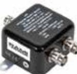
**VHF DIPLEXER SPLITTER**- Splits the signal from a VOR NAV antenna into NAV and glide slope receivers. Application: Navigation & Glide Slope Frequency: 108-118 & 328-335 MHz Impedance: 50 Ohms Nominal Connector: (3) Type "BNC" Females Max Weight: 3.5 oz Filtering: 30 dB Min / 40 dB Avg Insertion loss: 1 dB Maximum Isolation: 38 dB Min Dimensions: 2" x 1-3/3" x 1-1/8" RF Power Capacity: Receive only P/N AV-570 ..... **\$124.75**
