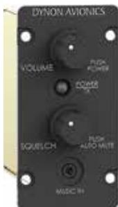
For ALL experimental and light sport aircraft. Ample inputs for EFIS systems, stereo music, and all the other technology in your panel. High-Fidelity Audio Circuitry, Dual Radio Support, Fail-safe between the pilot headset, Horizontal and Vertical faceplates are both included; headset jack kits also included. Selectable Auto Mute, and Independent intercom Voice Activation.
