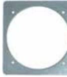
The G5 adapter plate is fabricated from 0.050 thick 2024-T3 aluminum per the dimensions shown in Figure 4-11. Apply a finish coat of paint to adaptor plates as desired prior to final installation. These may be field fabricated if needed and must have some type of corrosion protection (primer, alodine, etc.).
