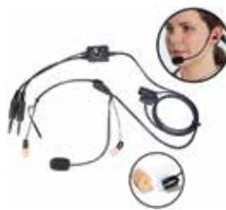
Used to improve both hearing protection and speech communications. Each earpiece includes a miniature speaker that reproduces speech signals from the aircraft audio system. The replaceable compliant foam tips attach to the earpiece and contain a pathway for the sound to travel from the transducer to the ear. Provides
