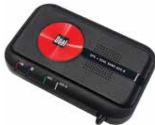
The XGPS 170D features a WAAS GPS and dual band (978/1090 MHz) ADS-B receiver for weather & traffic information. The receiver works with many EFB apps. It connects to up to 2 devices via Bluetooth, and is compatible with iPad, Android and Windows tablets. The internal battery lasts up to 5 hours of continuous operation, and the receiver can be charged with the included 12–30V adapter and wall charger. A non-slip pad is also included for convenience.
