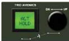
**EZ-3 ALTITUDE CONTROL** - The EZ-3 incorporates all of the features of the EZ-2 and adds the ability to pre-select a destination altitude. Once engaged, the system will initiate a climb/descent to the target altitude at a vertical speed that the pilot has previously specified.
