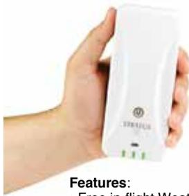
Stratus 3 is the simple-to-use, portable wireless receiver that provides subscription-free weather, GPS information, backup attitude and ADS-B traffic — integrated with ForeFlight Mobile for your iPad, and now including GDL 90 protocol to work with other flight apps.
