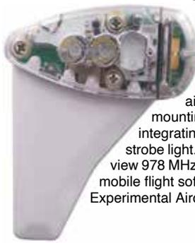
The skySensor EXP is the ADS-B in companion to the skyBeacon ADS-B out solution. This experimental-only wingtip ADS-B in receiver provides an easy to install path for dual band ADS-B in. The skySensor replaces your existing aircraft position light and uses the existing mounting location, breaker, and wiring while integrating an LED Navigation and Anti-Collision strobe light. The Wi Fi signal generated allows you to view 978 MHz and 1090 MHz traffic within your existing mobile flight software.
