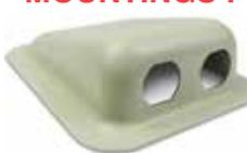
Metal housing available in raw Aluminum, Black or Beige. Designed to be utilized with the BOSE 6 Pin Lemo Jack #323172-0010. Can mount with (4) small screws on outer flange. Dimensions: W2.9" x L3.56" x H1.06". Weight: 22 grams. Note: Hardware not included.
