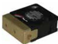
The SAFE 128 is an axial fan that is designed to attach directly to an avionics unit's cooling port. Providing a nominal 20 CFM (no load) of cooling air. The SAFE 128 provides an alert output whenever the fan RPM drops below a preset level.
