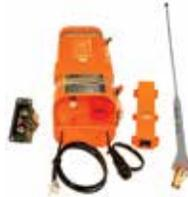
The all new E-04 ELT is a direct replacement for the more than 62,000 model E-01 ELTs (by ACK) on the market today. The new E-04 fits directly into the current E-01 mounting trays and uses the same remote control panel indicator. The E-04 external antenna will utilize your current antenna mounting and wiring installations.
