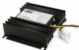
This unit is a step down voltage converter that drops 28 volts DC down to 13.8 volts DC. This unit would be required to operate either our COM 760 TSO or INS 422 TSO units in an aircraft or vehicle that are 28 volts DC. Specifications: • Physical Dimensions: L 4.0" (10.16 cm) x W 4.625" (11.75cm) x H 1.250 (3.18cm) • Weight: 0.75 lbs • Power Requirements: Current 2.0A Continuous with 5.0A Intermittent
