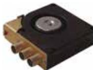
The SAFE 328 is a three port blower that can effectively cool a complete avionics suite. Providing a nominal 20 CFM of cooling air (no load), the SAFE 328 provides an alert output should the blower RPM drop below a preset level.
