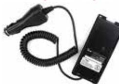
The CBE-210 is a DC battery eliminator for ICOM handheld radios such as the IC-V8, F3GT, F4GT, & F21GM. One end plugs into a 12-13.8VDC lighter socket. The coiled cord links the lighter plug to the battery housing, which clips onto the back of the radio. The CBE-210 includes Voltage & Current-limiting circuitry; noise filtering circuitry is also built into the housing. 5A fuse is located in the Cig Plug.
