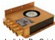
The ACF528 is a FAA-PMA'd five port cooling fan that produces cooling air for one to five avionics units. Supplying up to 20 cubic feet of air per minute at 28 Vdc, the ACF528 can easily cool an entire stack of avionics. The ACF528 uses a brushless blower motor to provide years of reliable RunQuiet™ operation.
