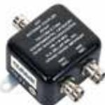
**VHF DIPLEXER COUPLER** - Splits the signal from a single antenna into two NAV receivers; eliminating the need for a second antenna. Application: Navigation Frequency: 108 to 118 MHz Impedance: 50 Ohms Nominal VSWR: 1.4 to 1 Maximum Connector: (3) Type "BNC" Females Max Weight: 3.5 oz Insertion loss: 3 dB Avg / 5 dB Max Isolation: 30 dB Minimum Dimensions: 2" x 1-3/3" x 1-1/8" RF Power Capacity: Receive only P/N AV-547 ..... **\$116.75**
