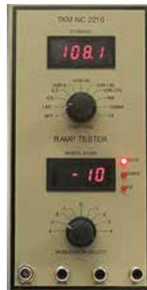
The NC 2210 Tester is optimized for ramp testing of navigation and communication equipment. The unit provides test signals for marker beacon, communication, localizer, glide slope, and VOR. Also included, is a wide band comm receiver to permit evaluation of comm transmitter AM fidelity. The TKM NC 2210 is a NAV-COM Ramp Tester. The unit has improvements over the 2200, which it replaces. The improvements include the following features:
