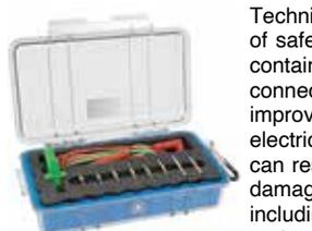
Technicians can work with a higher degree of safety when using the PIN-TS KIT. This kit contains the correctly sized tools for successful connector pin-testing without the need for improvised testing methods with uninsulated electrical contacts or the wrong size of pins that can result in electric shock to the user or lost/damaged pins. This kit has all of the essentials including insulated test leads, a ground lead, and two sets of four screw-in pins.
