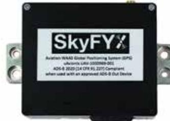
SkyFYX combines a high precision WAAS GNSS sensor with an integrated RAIM processor. Resilient against jamming, spoofing and GPS range errors—SkyFYX provides reliable navigation in challenging environments. SkyFYX is the most affordable ADS-B rule-compliant position source companion for the echoUAT ADS-B transceiver. The SkyFYX meets the performance requirements of 14 CFR 91.227. For use in Experimental and LSA aircraft.....P/N 11-15206 .....\$687.00
