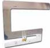
**MODEL 2** - Tail cap Com antenna for metal (conductive) airplanes installed inside a tail top fiberglass fairing with inside dimensions of at least 10" high x 12" long. VSWR is normally less than 2.0:1 over a COM frequency band of 118 to 136 Mhz.
