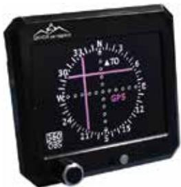
The SI-11X Electronic Course Deviation Indicator is a panel-mounted device that displays lateral and vertical needles from a typical navigation receiver or GPS navigator. The non-certified SI-11X CDI is intended for the experimental aircraft market.
