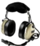
For rugged cockpit environments. Standard comfort features include protein leather covered dual density foam ear seals and washable polar fleece headpad • In-line quick disconnect jack on the mic boom for chemical defense suit and boom replacement • Dome-mounted volume control • DO-160D tested ? environmental and explosive proof • Passive noise attenuation 21dB NRR. Two-year warranty.....P/N 11-10395 ..... **\$269.95**
