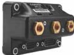
The GSU 25 is an Air Data Attitude Heading Reference System (ADAHRS) for aircraft flying up to 465 knots Indicated Air Speed\*.
