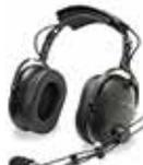
The 4DX Classic is an entry-level headset with classic Flightcom ruggedness. With an easy-to-position wire articulated boom and a ventilated foam rubber headpad and combined liquid and foam ear seals, the 4DX Classic is comfortable and affordable. Noise canceling electret microphone • Single-volume control • Stereo/ mono switchable • NRR 24dB • Weighs 16.9 ounces • Mic muff and cloth ear seal covers included • Three-year warranty P/N 11-17110 ..... **\$113.80**
